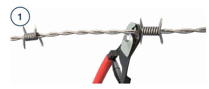
Cut wire at the barb, leaving at least 8 cm / 3 in of wire to make the join.
