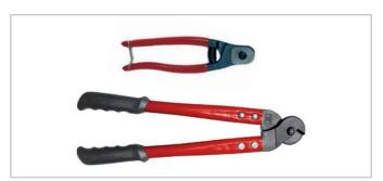
Wire Cutters are suitable for cutting high tensile wire or wire rope. Available in two sizes: up to 4 mm diameter and up to 6 mm diameter.
