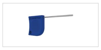
The Setting Key allows Gripple tensioners to be repositioned on the wire before tension is applied. To use, simply insert the key into the small hole adjacent to the main channel, releasing the roller and allowing the Gripple to move freely.
