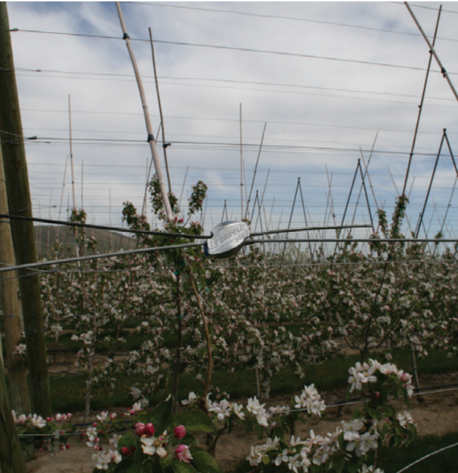
Gripple Plus Medium - Used to terminate trellising wire around a wooden post.
