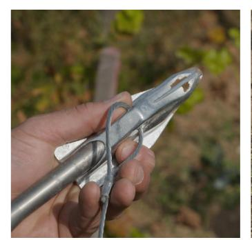
APEX anchor seated on Gripple Drive Tool.
